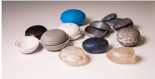
Figure 6. A collection of casing tests with 3D printed materials (sandstone, metallic plastic, resin, SLA), vulcanized plastic, silicone moulded surfaces, coated prints, and a natural stone.
